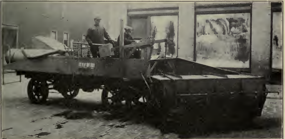
A ROTARY BROOM SWEEPER FOR CITY STREETS
